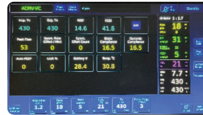
Screen 2 that indicates various parameters like MAP, RSBI Index, Static & Dynamic Compliance, Peak Flow, Battery voltage & other important parameters
